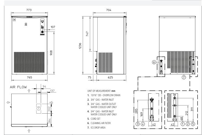
UNIT DATA SHIPPING DATA 773 x 704 x 1236 mm Size (W x D x H) Carton (W x D x H) Net weight 143 kg Weight
